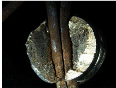
Third, the composition of the pin was not the bronze I believed it to be. In fact, the pin has a composition that is not typical of any marine alloy:
